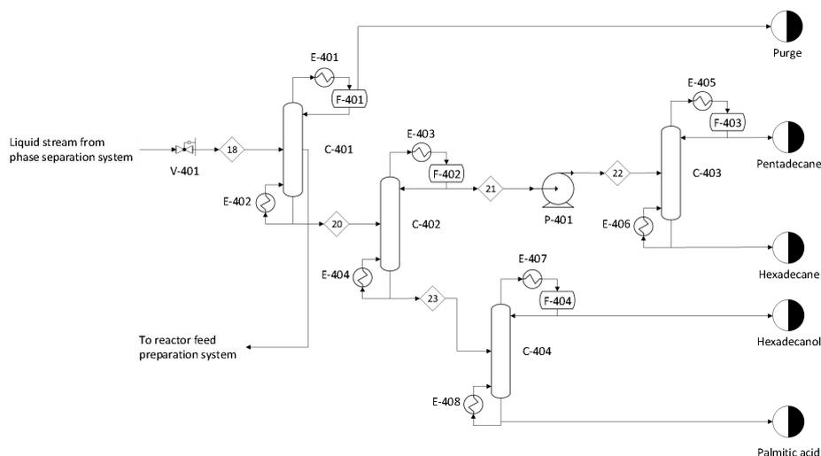
Fig.5 Process flow diagram of the phase separation system
