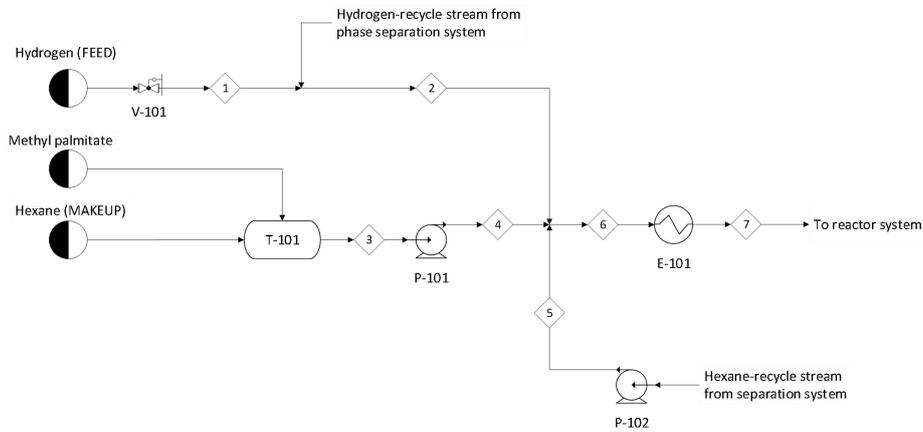
Fig.3 Process flow diagram of the reactor feed preparation system
