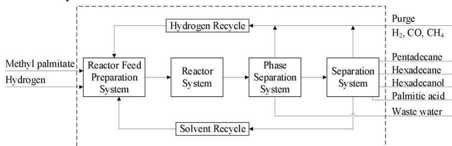
Fig. 2 Block Flow Diagram (BFD)
