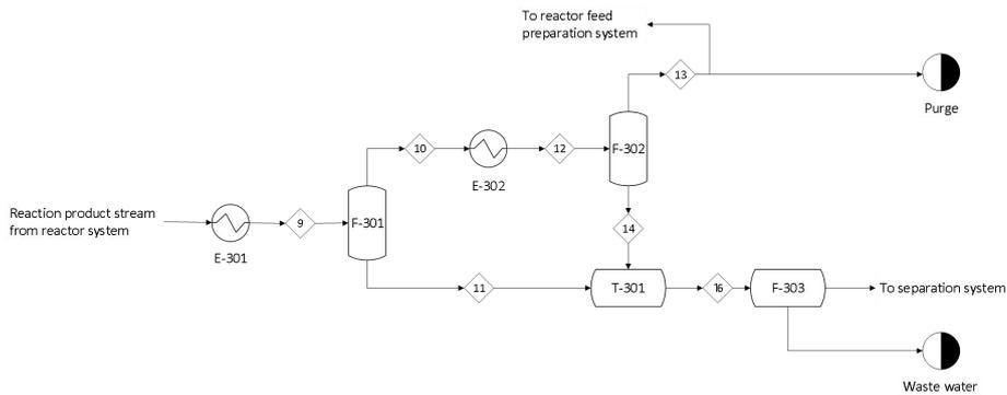
Fig.4 Process flow diagram of the phase separation system
