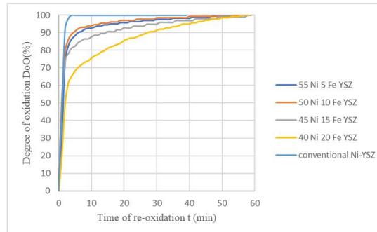
Fig. 2 Degree of oxidation (%) for Ni-Fe-YSZ compared to conventional Ni-YSZ in air atmosphere at 800°C
