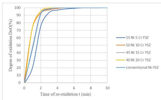
Fig. 3 Degree of oxidation (%) for Ni-Cr-YSZ compared to conventional Ni-YSZ in air atmosphere at 800°C
