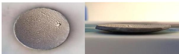
Fig. 5 The fabrication of hydrogen electrode using commercial NiFeCr-YSZ as a material
