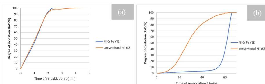
Fig. 4 Degree of oxidation (%) for Ni-Cr-Fe-YSZ compared to conventional Ni-YSZ in air atmosphere: (a) at 800°C, and (b) ramping from room temperature to 800°C
