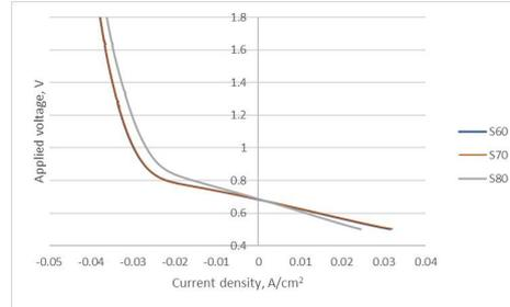
Fig. 6 Effect of steam to H<sub>2</sub> ratio (operating temperature at 800 °C)
