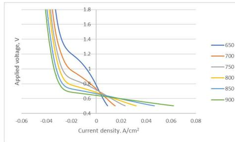
Fig. 7 Comparison of the electrochemical performance of various operating temperature and steam to H<sub>2</sub> ratio at 70:30
