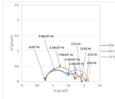
Fig. 8 Electrochemical impedance response of the Ni alloy wash-coated Ni-YSZ/YSZ/LSM-YSZ at different applied voltage at a constant operating temperature of 800 °C (H<sub>2</sub>O:H<sub>2</sub> = 70:30)
